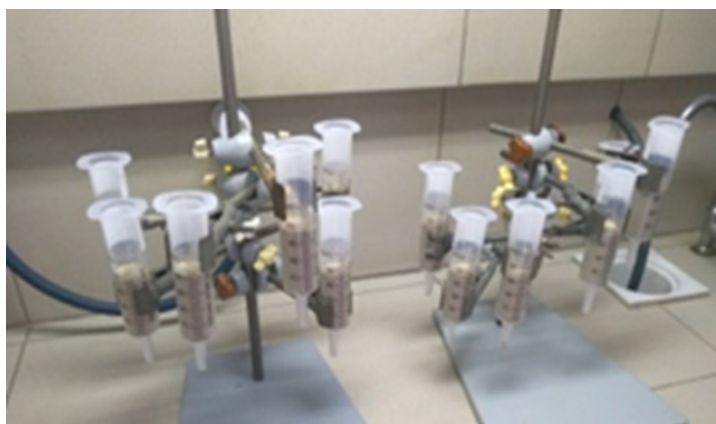
Figure 2. Sand columns for biocementation.
